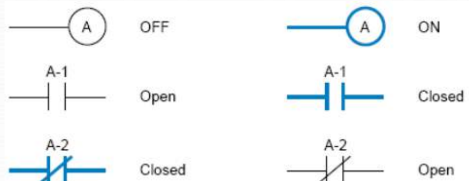
PLC Configuration for relay A
