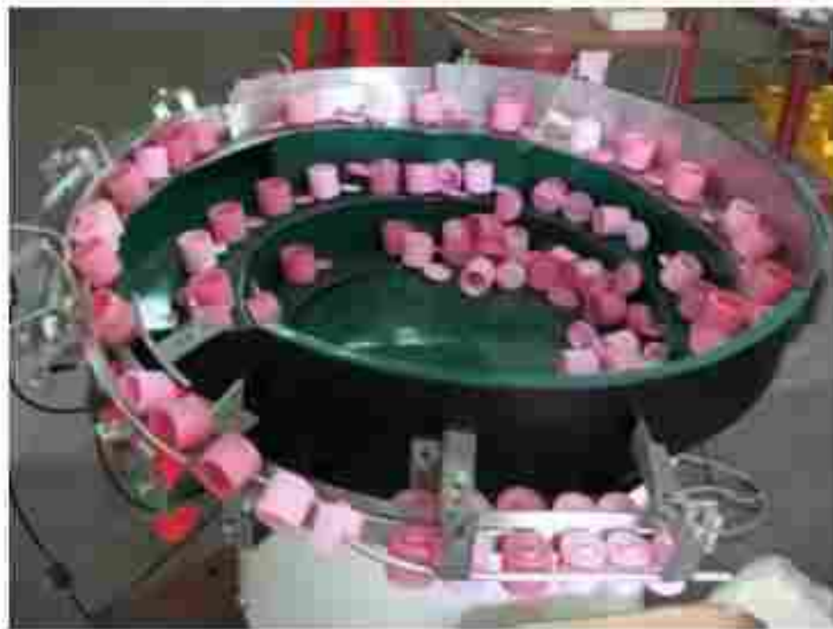
Figure (6.1b). Vibratory bowl feeder:
