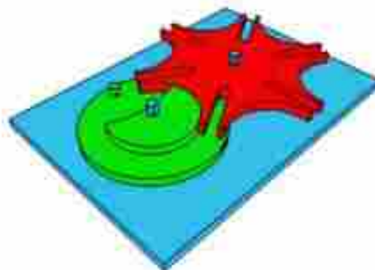
Figure (5.13b). Geneva mechanism
