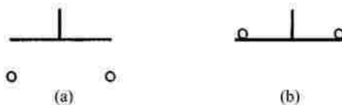
Figure (2.3). Momentary (spring-return) pushbutton: (a) Normally open; (b) Normally closed
